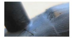
Closeup, showing the lines to the right of the valve, where the tube has developed leaks from being stretched too thin.
